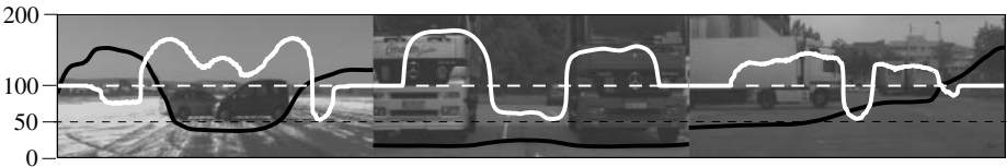
Fig. 5. Obstacle detection with distance histogram (black, scale on the left) and hypotheses verification (white, logarithmic scale, obstacle verified if above dashed line). The images show, that robust obstacle detection and verification is reached.
