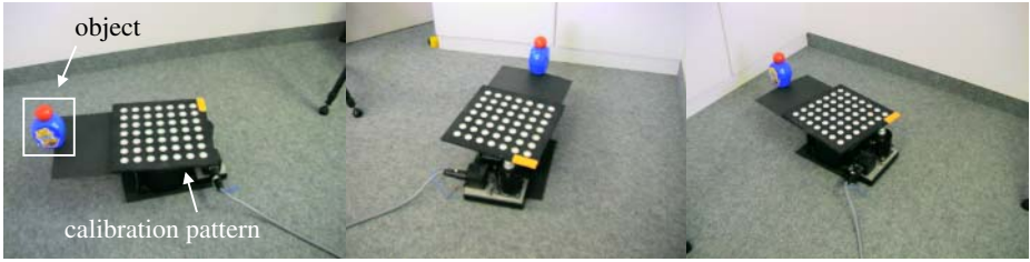
Fig. 4. The views of the test setup from all three cameras at the same time. The colored bottle is tracked as it turns on the turntable. The calibration pattern is used to initially calibrate all cameras, it is not used during tracking.
