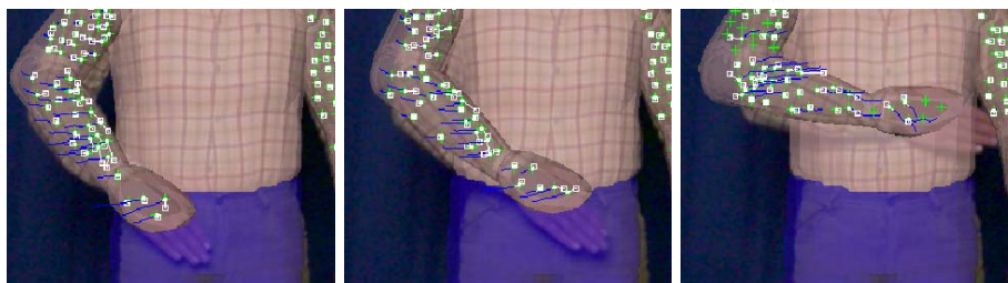
Fig. 2. Tracking of point features (Cross marks). Boxes indicate a tracked corner. The movement of a corner over the last frames is shown as a black line.
