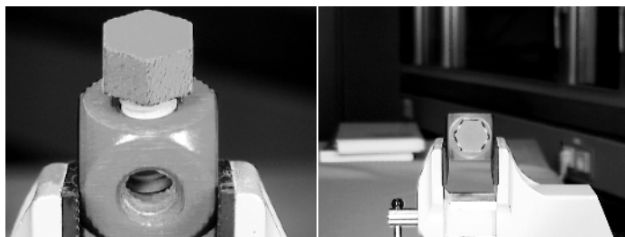
Fig. 1. A simple screw-block assembly. Left: Elevation 60^\circ , image scale 0.1 mm per pixel. Right: Elevation 0^\circ , image scale 0.3 mm per pixel.
