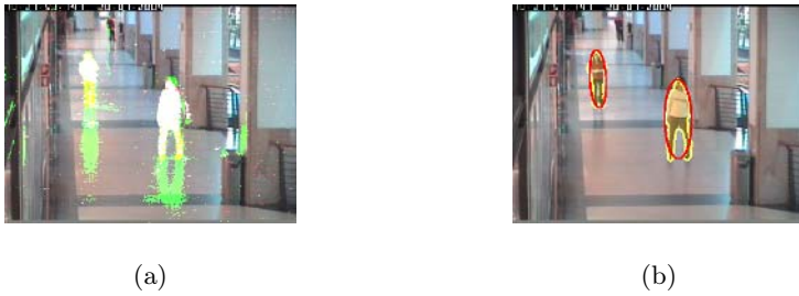
Fig. 2. (a) Segmentation: foreground pixels are painted on white, while those ones classified as dark foreground are on yellow, shadows on green, and highlights on red. (b) Detection: red ellipses represent each target, and yellow lines denote their contour.
