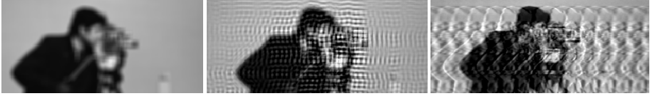
Fig. 3. Deconvolution with known PSF without using diffusion operator. Left: Blurred image. Middle: Deconvolution of Gaussian blur. Right: Deconvolution of motion blur.
