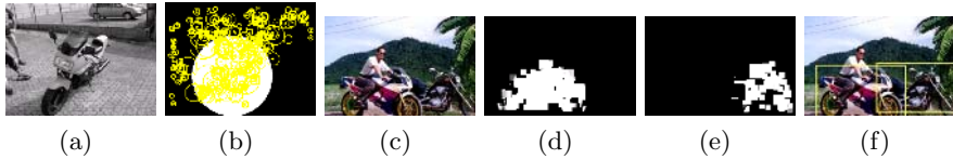
Fig. 3. (a) training image (b) estimated approximation of object segmentation (c) test image (d)+(e) inferred segmentation for hypothesis (f) final detections
