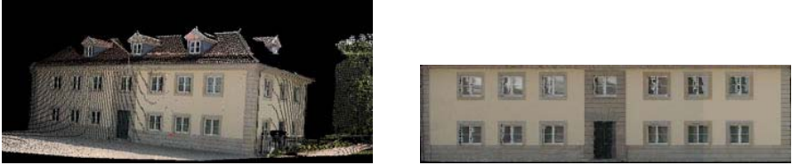
Fig. 1. Point cloud and orthorectified image of a façade
