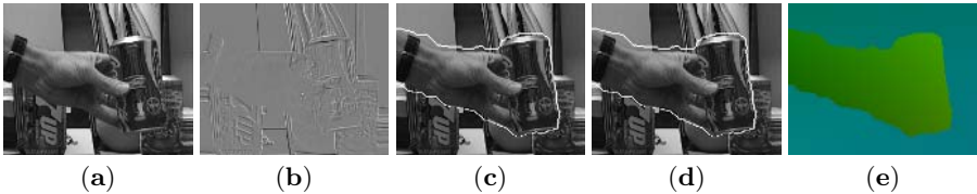
Fig. 6. Results for the Pickup Sequence (a) first frame (b) difference image to second frame (c) segmentation for the model with constant velocities, \nu = 3 (d) segmentation for the affine model, \nu = 3 (e) flow field for the affine model
