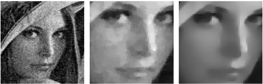
Fig. 5. Denoising. Left: Unblurred noisy image, SNR=8 dB, size: [256, 256]. Middle: TV method, PSNR = 27.1 dB. Right: Edge-driven diffusion, PSNR = 30.2 dB.
