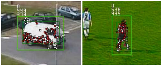
Fig. 3. A car and a soccer player with their current interest points (in white) and model points (in red) superimposed
