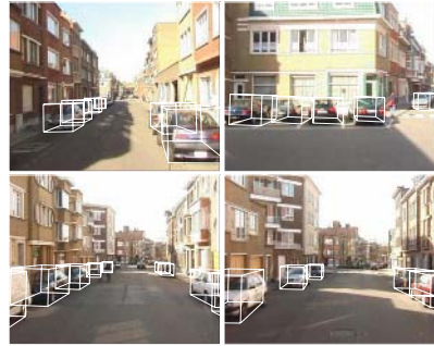
Fig. 8. (left) Comparison of the detection performance with and without scene geometry constraints. (right) 3D car location estimates using also information from future frames.
